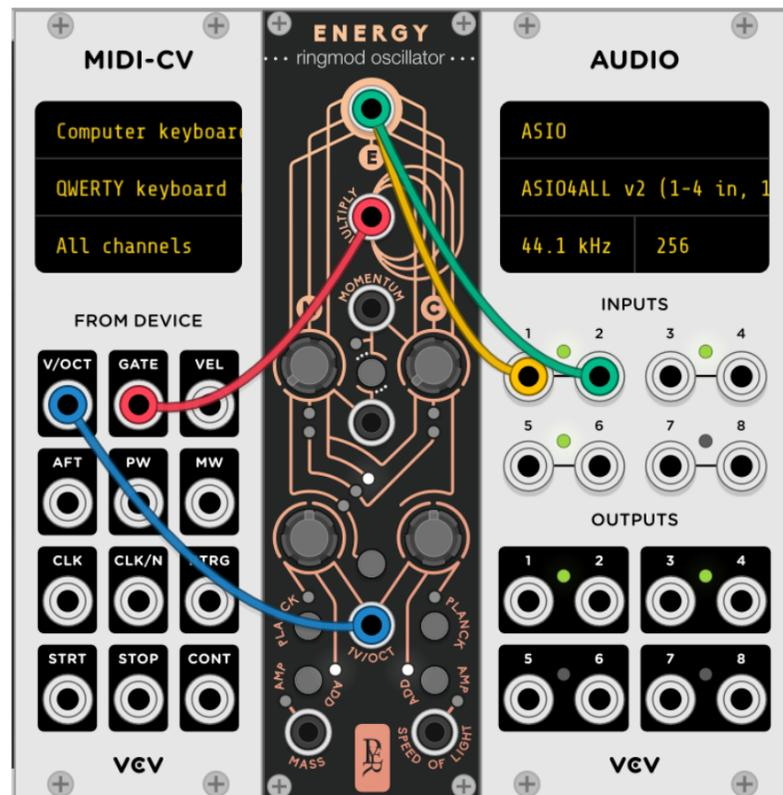
**Minimal synth voice:** a gate input can be directly connected to the multiply input, thanks to the soft slew limiter.
