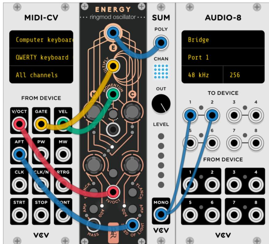
**Polyphony:** Energy can be turned into a 16 voice polysynth when a poly cable is connected to the v/oct input. All the CV input are poly-compatible to control each voice separately
