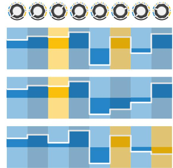
The probabilities for each step can be controlled all together by the **knob on the top**, which will add an offset to each knob. This knob is CV controllable with a -5V to +5V range.
