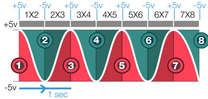
**A triangle wave** will make linear crossfade, while a **sinus wave** will create an exponential cross-fade
