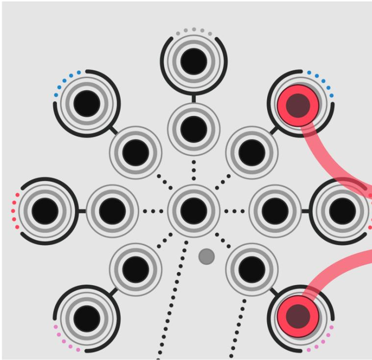
When no trigger or input source is connected: The outputs are just noise sources, different kinds of noise for each.
