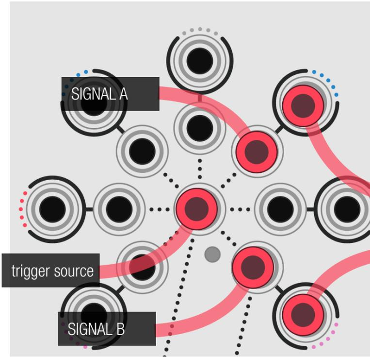
When a trigger and an input are connected, the noise generator is bypassed, and the S&H uses the input as material.
