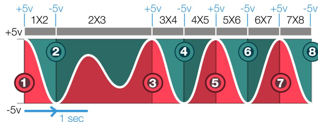
**Modulating the amplitude** of the signal can create some interesting rhythmic effects as it only switches to the next step when it reaches +/- 5 volts.
