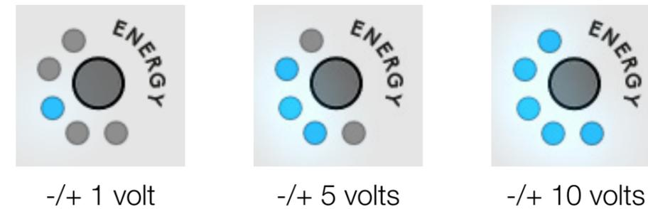
When the Planck constant is ON, IONS is a chromatic sequencer with Energy defining the range of CV:
