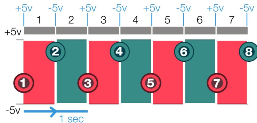
**A square wave** won't create a cross fade effect, it can then be used as a standard sequential switch.
