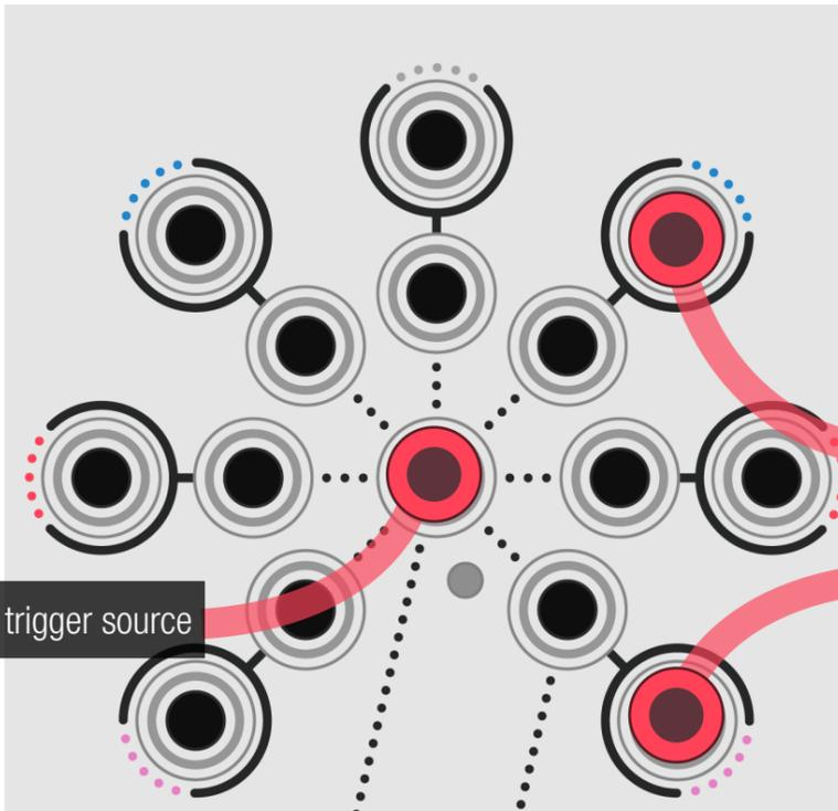
When a trigger is connected, the outputs use the trigger to sample and hold their internal noise generator and send random CV.
